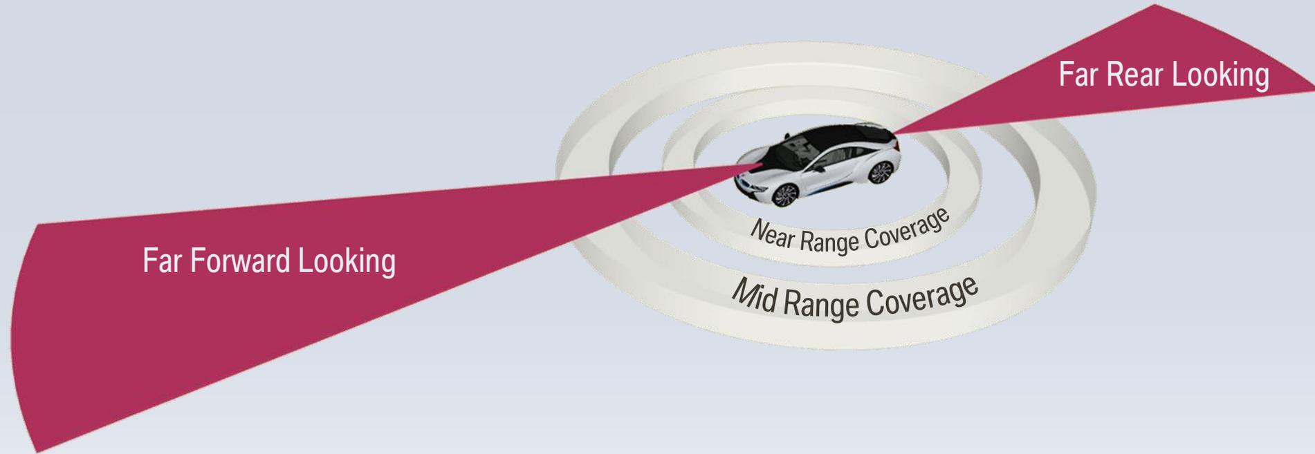
Redundant Sensor Coverage Per View
